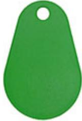
A green 45mm x 30mm x 2.2mm keyfob containing a MIFARE DESFire EV2 4K chip. This extremely durable, 100% waterproof thin keyfob is designed to be attached directly to a keyring. A useful alternative for contactless systems, it operates at 13.56 MHz wireless frequency, according to the ISO 14443A standard with the transport protocol complying to the ISO 14443-4 standard.
